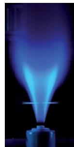
Stratified flame passed by laser beams for laser Doppler velocimetry (LDV) measurements
